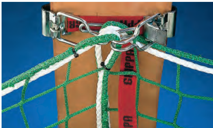
The two flange grips encircle the I-beam and are closed by pulling a strap with a snap lock.
