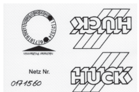
Test badge showing identity number and next inspection date. 4
