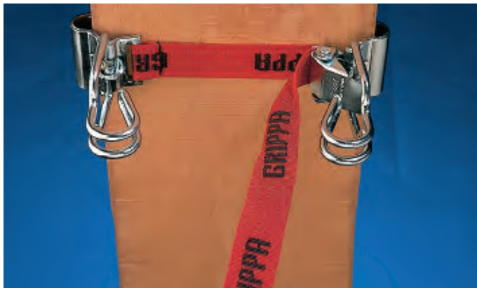
Hanging the edge rope in the hook (see photo) on the underside of the flange grip in a twisted position prevents unintentional detachment of the net.
