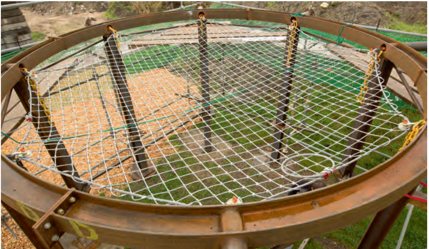
Wire rope net DRALO "Xtreme" in test framework.
