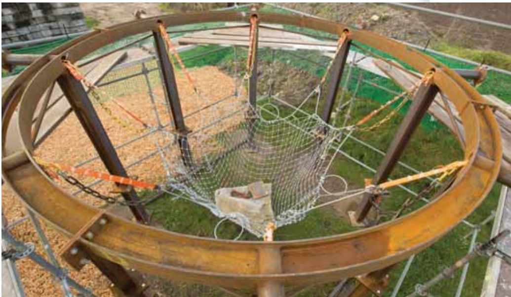
Actual condition following the drop test, with triggered "absorbers" Test body was an irregular-shaped boulder. Weight: 685 Kg, height of drop: 7.50 m
